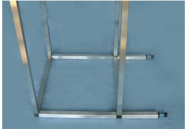
Lay the first frame on a firm flat floor. A sheet of cardboard or similar should be used on the floor to prevent scratches to the frame. Using a soft faced mallet, bang the four long tubes onto the projections as shown above. Place the other end frame on top and align the four tubes/projections. Drive the top frame onto the tubes by banging each corner down in turn about 10mm at a time until all tubes are seated onto the shoulders.
