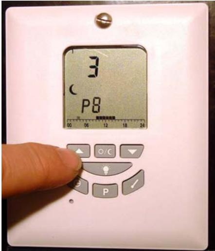
When the display has returned to normal press the P button three times to access the P8 program. Now use the UP arrow button to step through the program. The moon icon will appear wherever there is a blank block and the sun icon will be on where there is a solid block.
