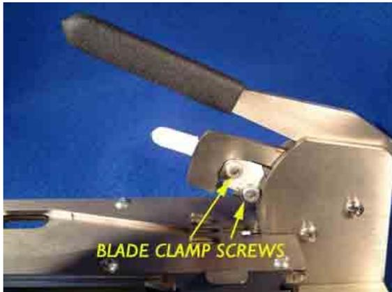
Changing the blade is not a regular task because blades last a long time on normal moisture content grain. The first time you change a blade it may be a good idea to completely remove the clamp screws and the blade clamp plate to see the blade location shim and understand how it locates the blade into a specific position. Replace the clamp plate and tighten the screws without the blade in place. You can now proceed as if it was a normal blade change.
