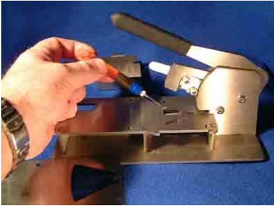
The bed plate should be oiled all over with a THIN film of oil (5 or 6 drops of oil smeared around with a finger tip) and the shim plate aligned on top
