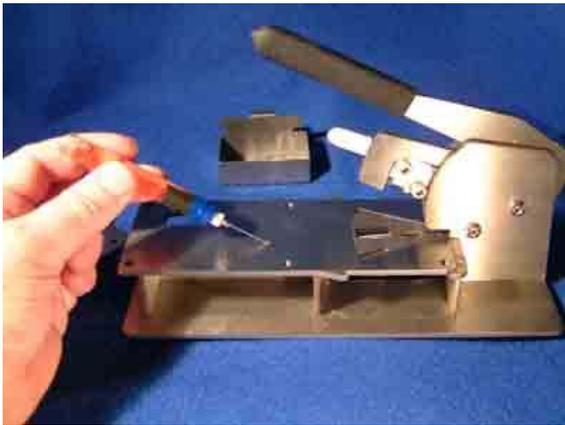
A thin film of lubricant should also be smeared on the top face of the shim plate to prevent the risk of moisture ingress.
