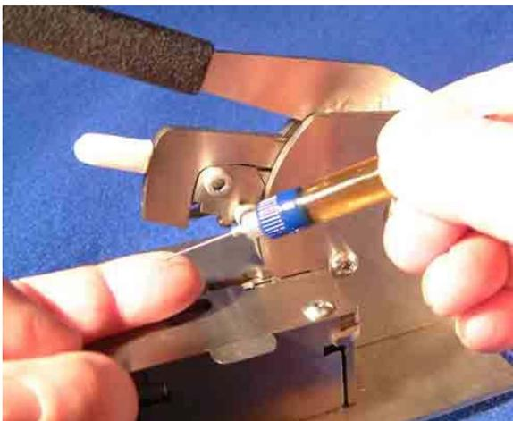
For heavy users "tooth" lubrication should be done approximately every 2000 operations (40 to 50 tests)
