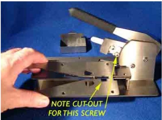
Slide the top plate into alignment with the other plates and drop the 6 screws back into position. Screw the 6 fixings in about 2 turns each to ensure full alignment of all plates and then fully tighten all screws.
