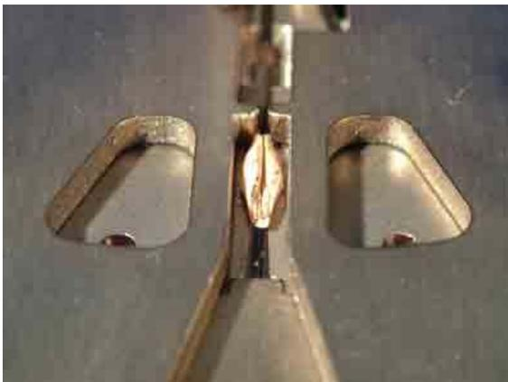
To achieve good splitting it is desirable that the germ end of the grain is slid into the small slot in the end stop. This guarantees the germ is centrally split even if the rest of the grain is not aligned properly. Experience has shown that the "V" shaped clamp will usually pull the grain into good alignment and symmetrical splitting will occur even if the germ end is not against the end stop.
