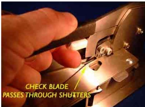
When the blade has been fitted, take a few seconds to carry out this simple check to ensure correct functionality. Lift the "V" clamp clear of the blade with the white handle and check that the blade passes into the gates before they start to open.
