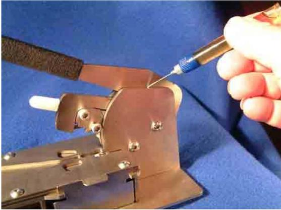
For both heavy and light users, 3 or 4 drops of oil each side of the operating lever each WEEK will be adequate.
