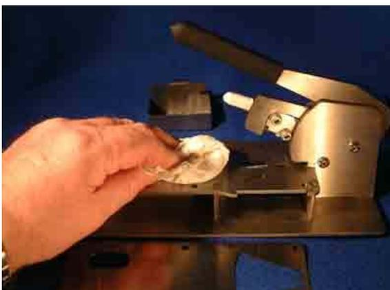
Remove the shim plate and wipe it clean. Note the shim plate is not stainless and some additives in certain oils may cause staining.
