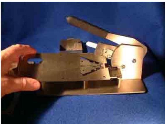
Carefully remove the shutter plate and place it on a clean flat surface before disassembling the shutters and springs. The polymer springs are circular when new but after a short time take up a distorted shape close to their assembled "squashed" shape. This does NOT impair their effectiveness.
