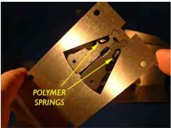
After cleaning, reassemble the shutter plate, making sure that the polymer springs are in the correct slot and pushed flush/sub-flush to the surface. Assemble and align it on top of the shim plate.
