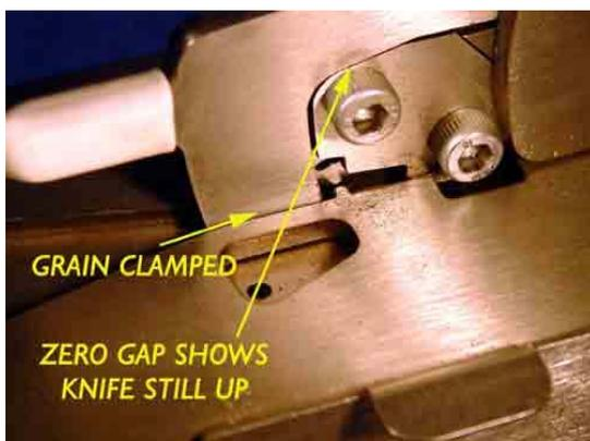
When the operating lever is pulled down there are three distinct phases to the cutting cycle which can be felt. The first resistance is felt when the "V" clamp aligns and locks the grain. At this point the knife has still not yet started cutting the grain.
