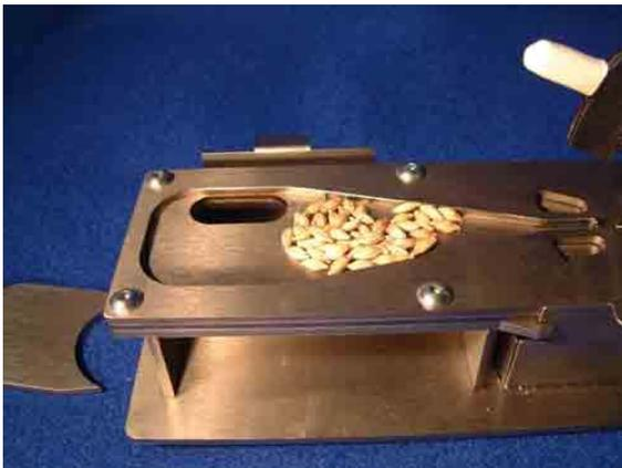
Provision to clear any residual test grains has been made. One of the sample trays can act as a collector tray.
