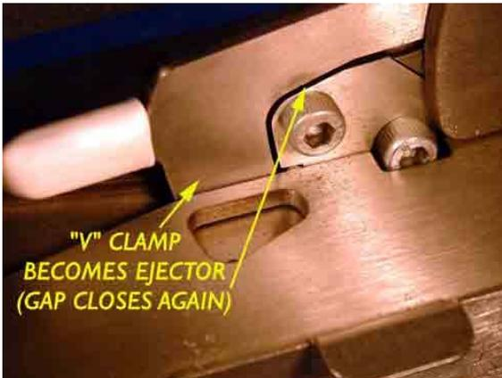
Further pressure on the operating lever opens the shutters and allows the sprung loaded “V” clamp to pass through the shutters, thus acting as an ejector to send the split grain into the two collecting trays.
