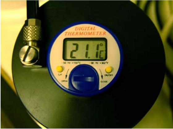
The thermometer continually monitors the temperature of the test fluid. It is a compact battery powered unit that turns it's display off after 10 minutes to conserve power. Typical battery life is about 5000 hours. One press of the ON/OFF button restores the display.
