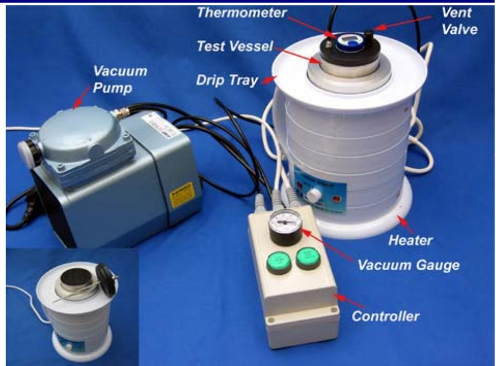
Testing malting barley (and other seeds) for a viable germ has never been simpler. This cost-effective solution has been developed in conjunction with end users to meet the need for fast turn-round testing in one space efficient unit.
